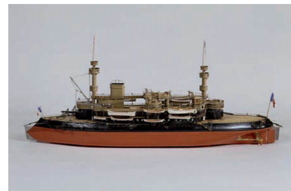
Hoche. Model of the squadron battleship launched in 1886. Lorient naval shipyard's model-making workshops, based on plans by Charles Ernest Huin (1836-1912). End of the 19 th century. Scale 1/66. Painted wood, steel, metal, brass and plant fibre. Inv.: 25 MG 16 © Musée national de la Marine/A. Fux
